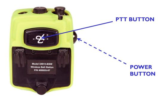
...then <u>release the PTT switch</u>. The LED indicator will <u>flash red</u> for 15 to 20 seconds, followed by a voice prompt, "Connection Deleted."
